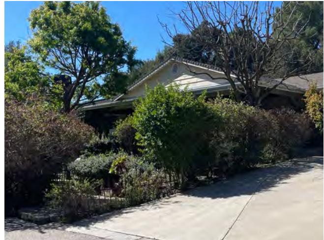
Figure 48: Overgrown vegetation in Zone 0 and 1 proximate to the exterior of the home. This introduces several paths for fire to spread and encroach the home.
