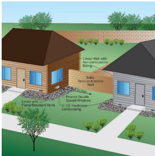
Figure 64. Examples of additional structural hardening and defensible space features where 30 feet of setback to the property line is not feasible (FEMA).
